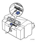
c Plug the other end of the USB cable into the USB port on the computer.
