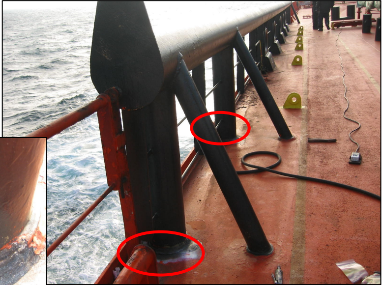
Crack in deck plating at hose saddle support (midship area)
