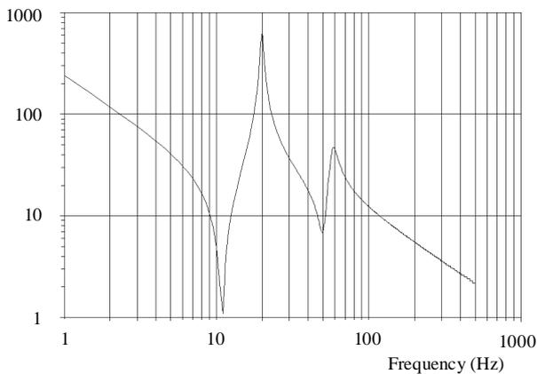
Figure 28. Example of a Transfer Function from Air-Gap Torque to Motor Speed for a Three Inertia Rolling Mill System.
