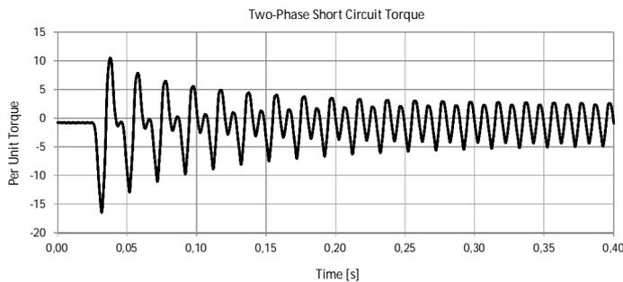
Figure 7. A Typical Two-Phase Short-Circuit Torque in the Air-Gap of a Motor.
