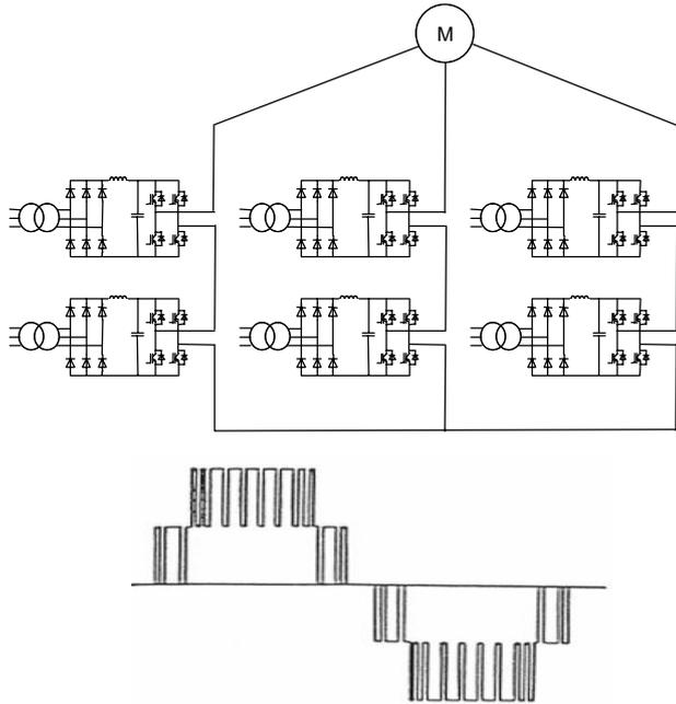
Figure 17. Five-Level Cascaded H-Bridge (CHB) Converter and Example of its Phase Voltage Waveform.
