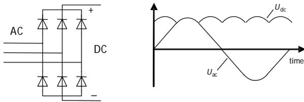
Figure 23. Six Pulse Rectifier and the Voltage Waveforms.
