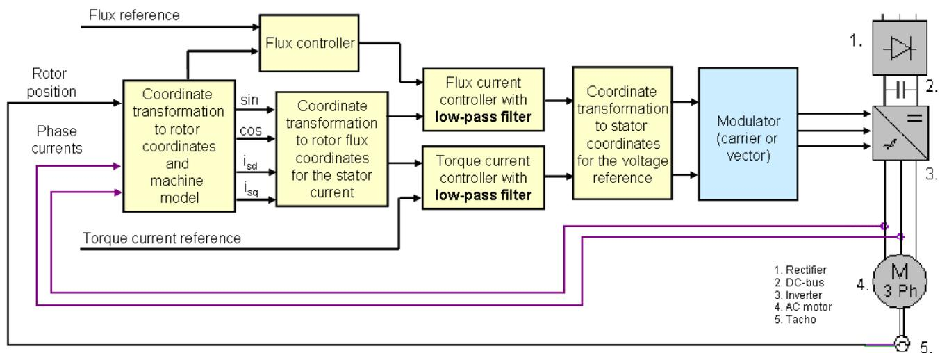
Figure 21. Rotor Flux Oriented Vector Control.
