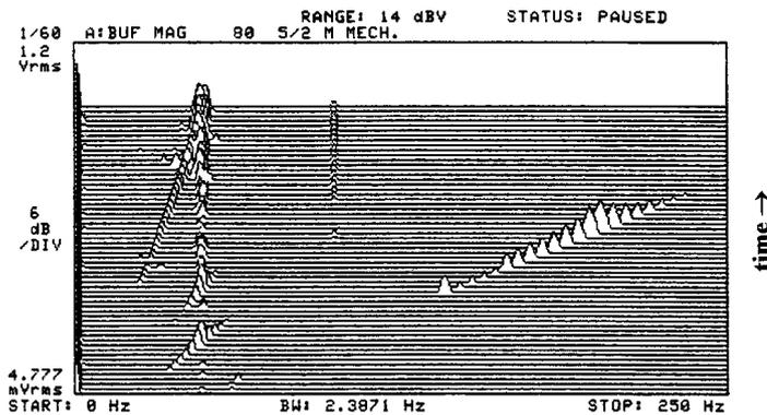
Figure 25. Example of the Shaft Torque Spectrum Variation when the Measured VSI Drive Was Accelerating. The Frequency of the Supply Network Was 50 Hz. Frequency Range of the Spectrum Analysis Was 0...250 Hz.
