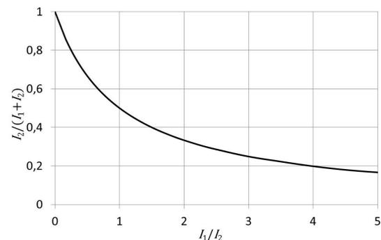
Figure 8. Effect of Ratio  $I_1/I_2$  on the Inertia Factor.
