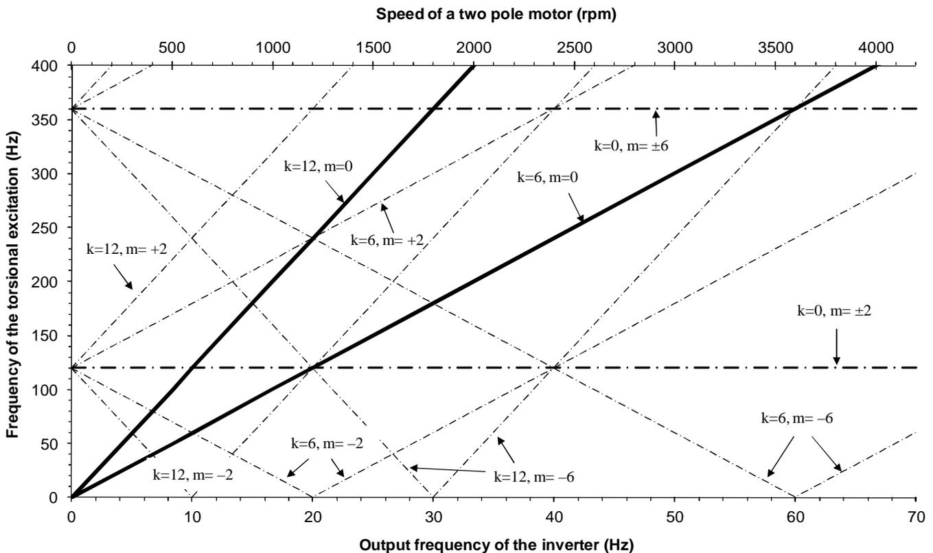
Figure 24. Most Important Harmonic and Interharmonic Excitation Frequencies of Motor Torque Represented on the So-Called Campbell Diagram when the Supply Network's Frequency Is 60 Hz.
