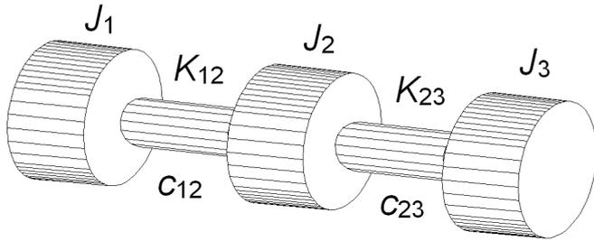
Figure 27. Example of a Drive Train Consisting of Three Moments of Inertia and Two Shafts with their Torsional Stiffnesses and Dampings.
