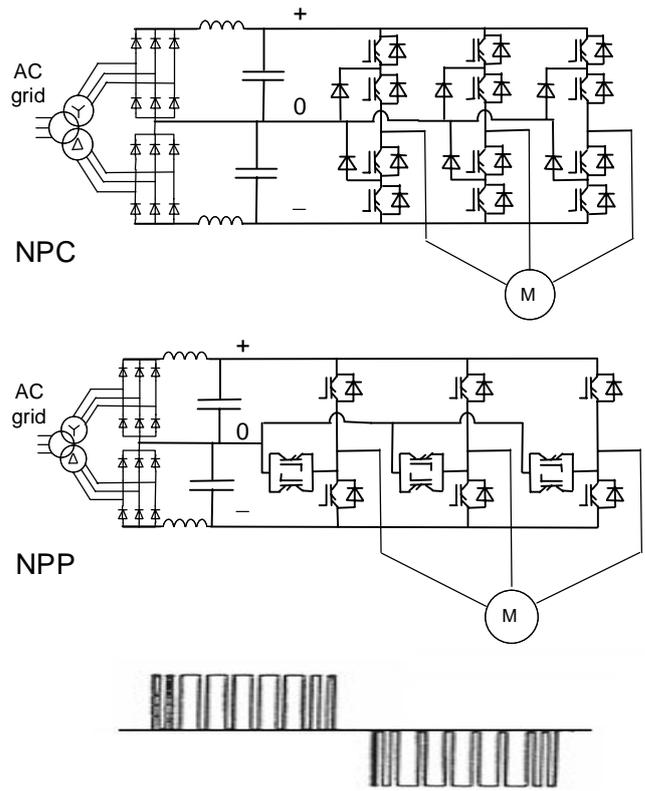
Figure 16. Examples of the Three-Level Voltage Source Converter Drives that Have Diodes in the Twelve Pulse Rectifier and IGBTs in the Inverter. Example of the Phase Voltage Waveform Is Also Shown. NPC = Neutral Point Clamped, NPP = Neutral Point Piloted.
