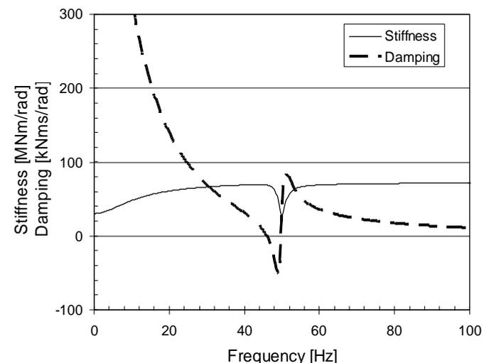
Figure 6. Torsional Stiffness and Damping of a 36000 hp Synchronous Motor with Supply Frequency 50 Hz (Holopainen et al. 2010).
