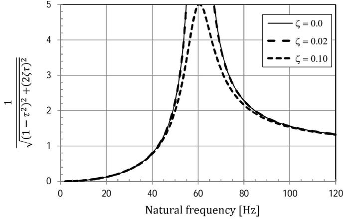
Figure 9. Dynamic Amplification Factor as Function of Natural Torsional Frequency with 60 Hz Excitation Frequency.
