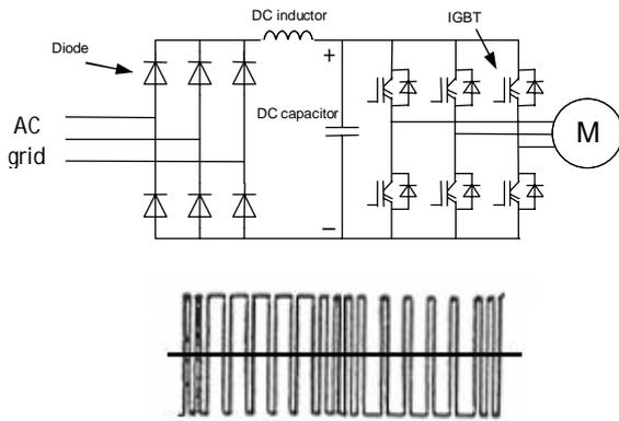
Figure 15. Two-Level Voltage Source Converter Drive that has Diodes in the Rectifier and IGBTs in the Inverter. Example of the Phase Voltage Waveform Is Also Shown.
