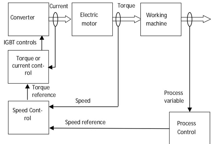
Figure 26. Block Diagram of Drive System Control.
