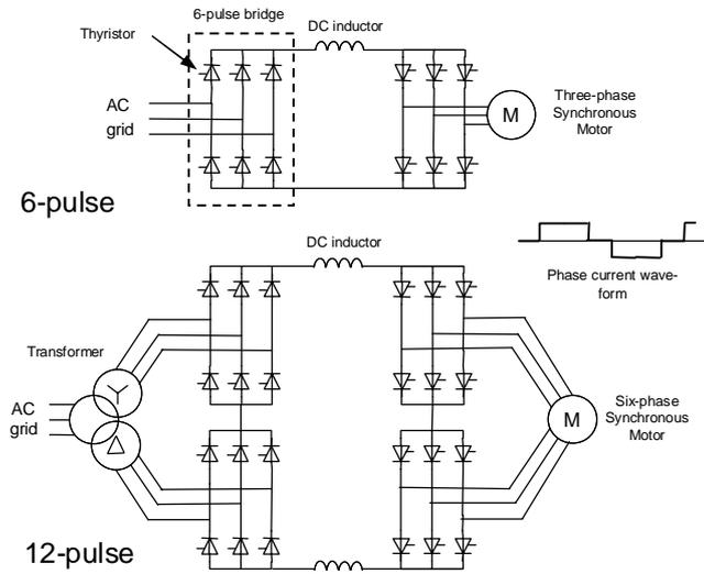
Figure 14. Six- and Twelve-Pulse Load Commutated Current Source Converter Drives and Their Ideal Phase Current Waveform.
