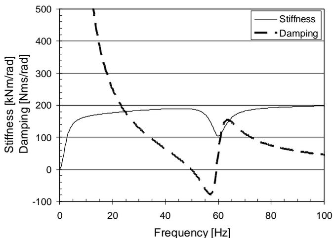
Figure 5. Torsional Stiffness and Damping of a 1250 hp Induction Motor with Supply Frequency 60 Hz (Holopainen et al. 2010).
