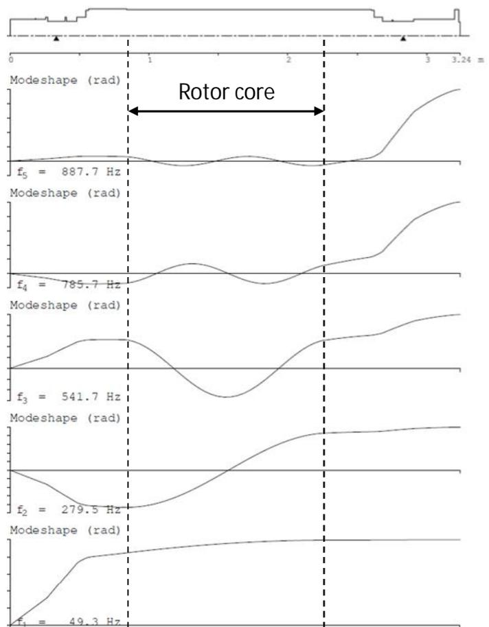
Figure. 3 The Five Lowest Torsional Modes of a Two-Pole 9400 hp Induction Motor with Rigidly Fixed Coupling End on the Left. High up, the Geometry of the Shaft without Rotor Core is Shown.
