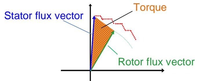
Figure 20. Torque Is Proportional to the Area of the Triangle between the Stator and Rotor Fluxes. The Path that the Tips of the Counterclockwise Rotating Vectors Have Traveled Is Shown with Dotted Lines.
