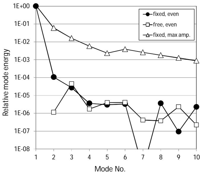
Figure 4. Relative Mode Energy in Resonance Condition Excited by an Evenly Distributed Unit Torque or by a Unit Torque in Maximum Modal Amplitude of the Core.
