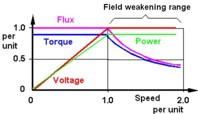
Figure 12. Attainable Torque and Power of a Typical Induction Motor Drive with Rated 1 Per Unit Current as a Function of the Speed. Magnetic Flux and Voltage of the Motor are Also Shown.
