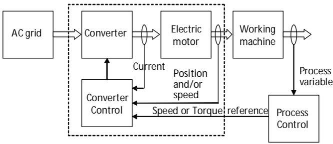
Figure 11. Structure of a Variable Speed Drive System.
