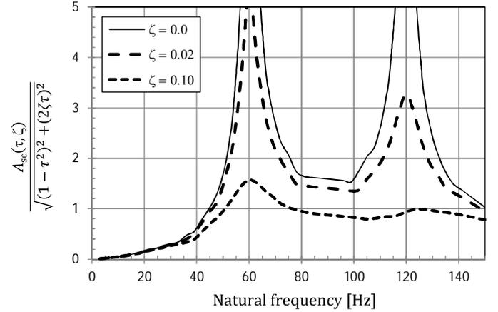
Figure 10. Amplification Factor for Transient Short-Circuit Load (DIN 4024) as Function of Torsional Frequency of the Lowest Mode with 60 Hz Grid Frequency.
