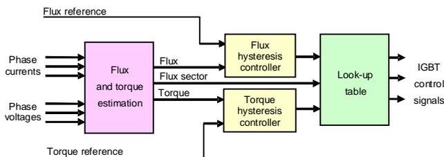
Figure 22. Principle of the DTC Control. (Courtesy of ABB)
