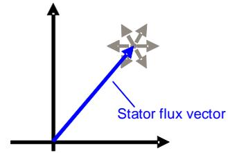
Figure 19. Influence of the Voltage Vectors to the Stator Flux.
