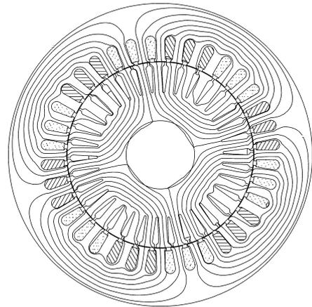
Figure 1. Magnetic Field of a Four-Pole 15 kW Induction Motor (Holopainen and Arkkio 2008).
