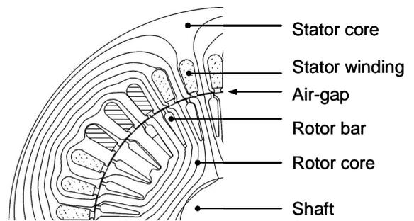
Figure 2. Main Parts in the Core Region of a Four-Pole 15 kW Induction Motor (Holopainen & Arkkio 2008).
