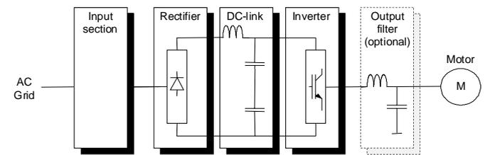
Figure 13. Structure of a Variable Speed Drive System.
