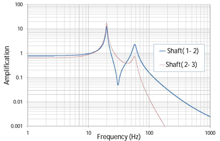
Figure 29. Example of the Amplification of the Air-Gap Torque Excitations Calculated for the Shafts of a Three Inertia Rolling Mill System with Same Parameters than in Figure 28.
