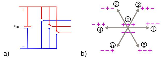
Figure 18. a) Two-level voltage source inverter represented as a set of switches, b) Voltage vectors that the inverter can output.
