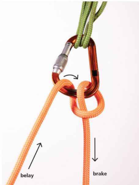
Figure 1-15. A munter hitch in the belay position on a locking carabiner on the anchor.
