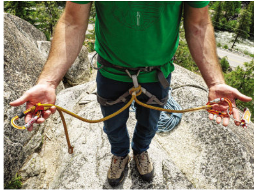
Figure 4-1. The Petzl Dual Connect is one of many prefabricated rappel extensions. It offers an adjustable-length clip-in point—the end in the climber’s right hand (the belay device is clipped to the other end)—and is dynamic, very durable, and heat resistant. While prefabricated options like the Dual Connect are dedicated tools, meaning you are “carrying something extra,” they serve their purpose extremely well.
