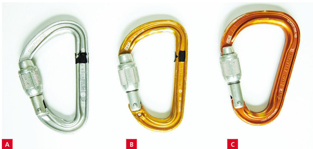
Figure 13-1. A variety of locking carabiners: a, lighter-weight; b, midsized that can still be used to adjust a clove hitch; c, full-sized HMS or pear-shaped.
