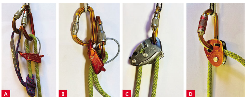
Figure 9-2. Different types of ratchets: a , belay device in guide mode; b , third-hand friction hitch (here, a prusik hitch) and carabiner; c , an assisted-braking belay device (ABD—here, the Petzl GriGri); d , a mechanical ratchet (here, the Petzl Micro Traxion).
