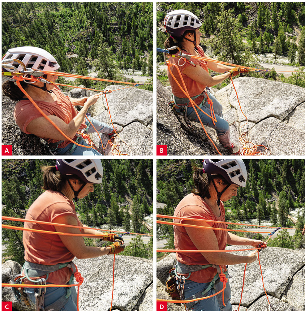
Figure 9-9. The 6:1 direct line haul from a belay: a, start from a 3:1 direct line haul with a backup clove hitch; b, tie a clove hitch on the hauling strand and clip it to a carabiner just above the lower friction hitch (prusik); c, clip the back-side strand of the clove hitch that backs up the system to the clove hitch you just tied; d, start hauling.
