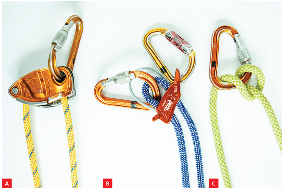
Figure 2-1. Belay options: a , the Petzl GriGri, an assisted-braking belay device (ABD); b , the Petzl Reverso, an autoblocking belay device; c , a munter hitch. (Photo by Truc Allen)
