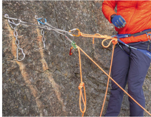
Figure 3-11. An overhand stopper knot (a.k.a. “catastrophe” knot) is tied 2–3 feet behind the belay device, so in the event the device were to be defeated, the knot would jam against the device, limiting how far the following climber would fall.
