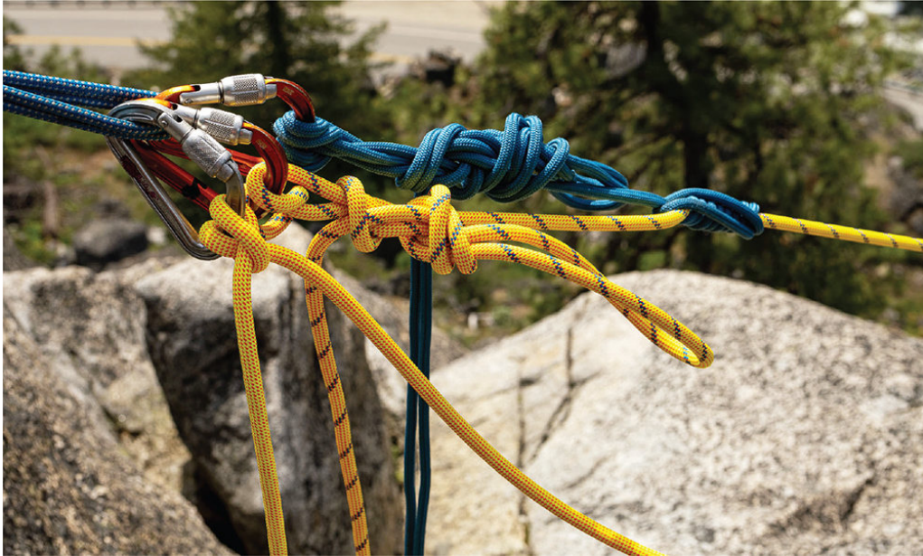
Munter-mule-overhand: among the most useful and most commonly used hitches for rock rescue, the munter-mule (tied on the striped yellow rope) can be tied off to create a load-releasable system—and it can be released even under tension. (Photo by Jim Meyers)
