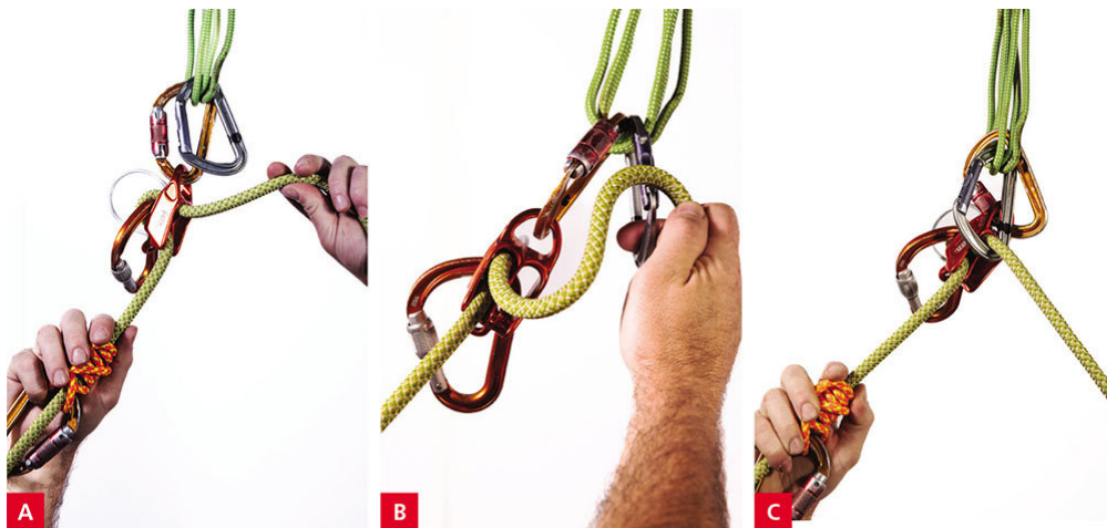
Figure 5-10. A load strand direct lower with an autoblocking belay device: a, put a third-hand friction hitch on the brake strand and clip a nonlocking carabiner to the anchor next to the locking carabiner the belay device is clipped to (on the side of the device where the brake and load strands exit, opposite the keeper loop); b, have the climber being lowered stand up to create a little bit of slack in the load strand, then clip the load strand to the nonlocking carabiner; c, with the nonlocking carabiner “defeating” the device, lower the climber while managing the friction-hitch backup.
