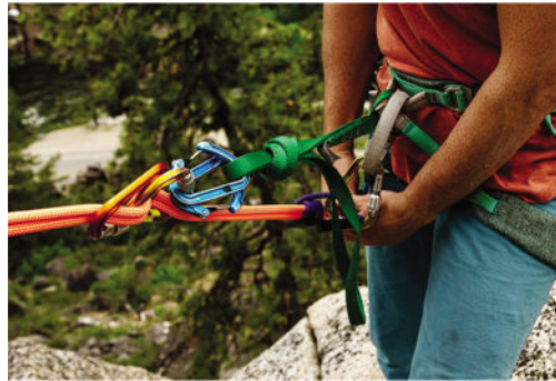
Figure 13-4. A double-locker rappel setup uses two locking carabiners to create friction for the rappel, plus two nonlocking carabiners opposite but not opposed as a backup. (Photo by Jim Meyers)
