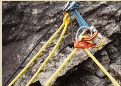
Using a 5.5mm cordelette for a classic plate release
