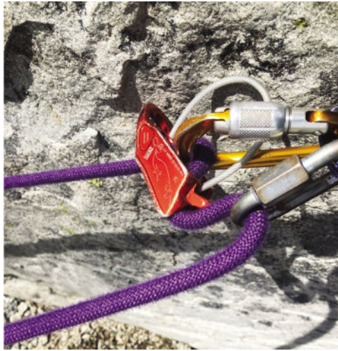
Figure 5-2. Redirecting through a fixed rappel anchor's chains: thread the end of the rope through the chains of a fixed rappel anchor, not only to use the lowest link to redirect the belay device but also to simultaneously pull the rope through the chains.
