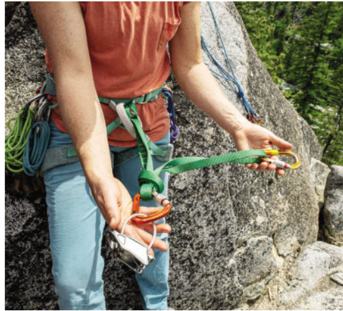
Figure 4-3. To fix the belay device carabiner in place, tie an overhand on a bight in the middle of the double-length sling; this setup provides slightly more redundancy but does not allow as much length for clipping anchors.
