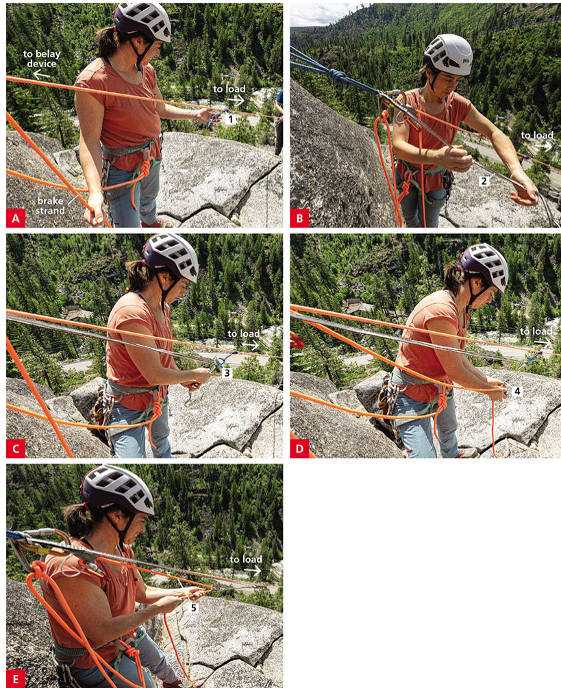
Figure 9-10. The 5:1 direct line haul from a belay: a, use a third hand or fairly short piece of material to tie a friction hitch (here, a prusik [1]); on the load strand coming out of the belay device; b, girth-hitch a long runner (2) to the anchor; c, clip the runner through a carabiner (3) on the friction hitch; d, clip another carabiner (4) to the runner's free (non-anchor) end; e, clip the brake strand (5) to this new carabiner and start hauling.
