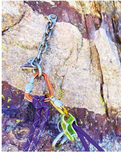
Figure 2-24. Two-piece anchor with a fixed rappel ring: this welded chain anchor by Fixehardware, which consists of two bolts connected with a welded chain and fixed rappel ring, is rated at 25–30 kilonewtons; the master point is the locking carabiner clipped to the ring. (Photo by Dale Remsberg)
