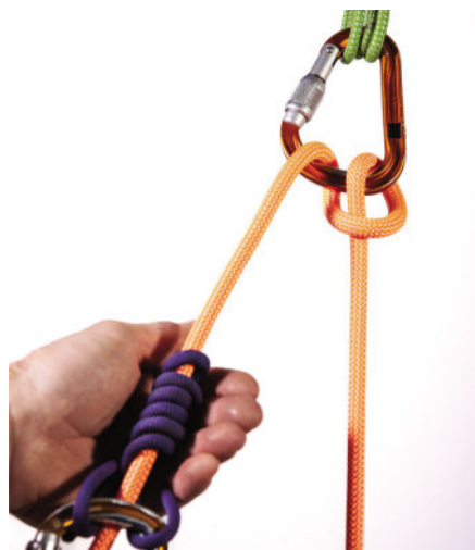
Figure 5-6. An HMS-style (pear-shaped) carabiner is wide enough to allow the munter hitch to easily flip back and forth during a lower, which will not only be easier to work with but also put far fewer twists in the rope. (Photo by Truc Allen)
