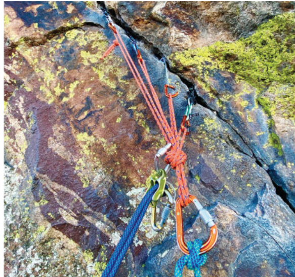
Figure 2-13. A four-piece anchor with the shelf used as another full-strength clip-in point: the shelf is secure and redundant as long as there is something clipped to the master point and all the individual loops of the shelf are clipped simultaneously. (Photo by Dale Remsberg)
