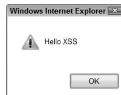
FIGURE 3-2: An example of a simple XSS attack
