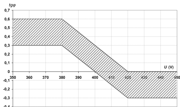
Fig. 1. Example of static Q(U) characteristic for DG prescribed in Slovenia [12].
