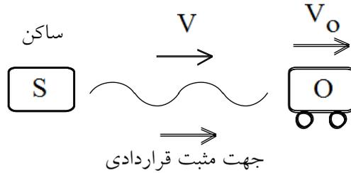
$$\frac{v_{o2}}{(+V) - (+V_o)} = \frac{v_s}{(+V) - 0} \Rightarrow \frac{v_{o2}}{V - V_o} = \frac{v_s}{V} \Rightarrow v_{o2} = \frac{V - V_o}{V} v_s < v_s$$
