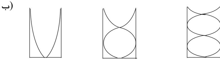
$$\text{پ) } \lambda_1 = \frac{V}{v_1} = \frac{340}{60} = 5/67 \text{ m} \quad \lambda_2 = \frac{340}{180} = 1/89 \text{ m} \quad \lambda_3 = \frac{340}{300} = 1/13 \text{ m}$$
